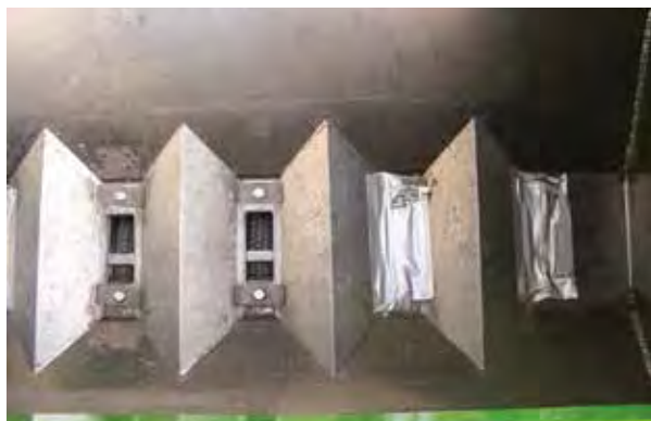
Figure 6. To create an alternating row configuration, duct tape is used to seal off openers in the large (top) and small (bottom) seed boxes of a grain drill. The resulting pattern will plant two rows of the varieties in the large box alternating with two rows of the varieties in the small box.
